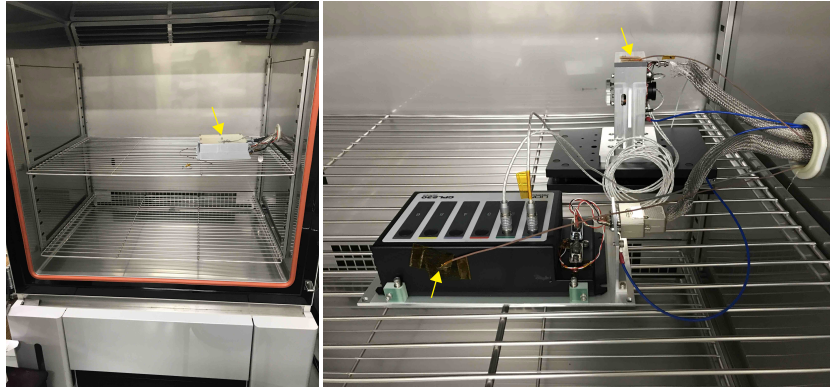
Figure 12. Photograph of the SMM-DRV, and SMM-TM together with SMM-IF, placed inside the thermal chamber with its door opened. Yellow arrow indicates the location of the attached thermocouples to monitor the temperatures of each SMM component.
